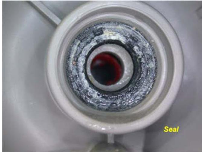
10. Whirlpool has known for at least eight years that the Dishwashers contain one or more design and/or manufacturing defects, including but not limited to the defectively designed and manufactured sump assembly with the inversely oriented Diverter Shaft Seal in the Class Dishwashers.
