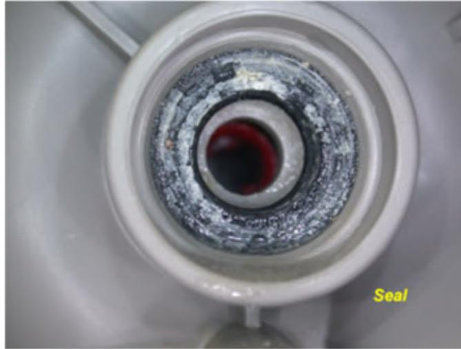
10. Whirlpool has known for at least eight years that the Dishwashers contain one or more design and/or manufacturing defects, including but not limited to the defectively designed and manufactured sump assembly with the inversely oriented Diverter Shaft Seal in the Class Dishwashers (“the Defect”).
