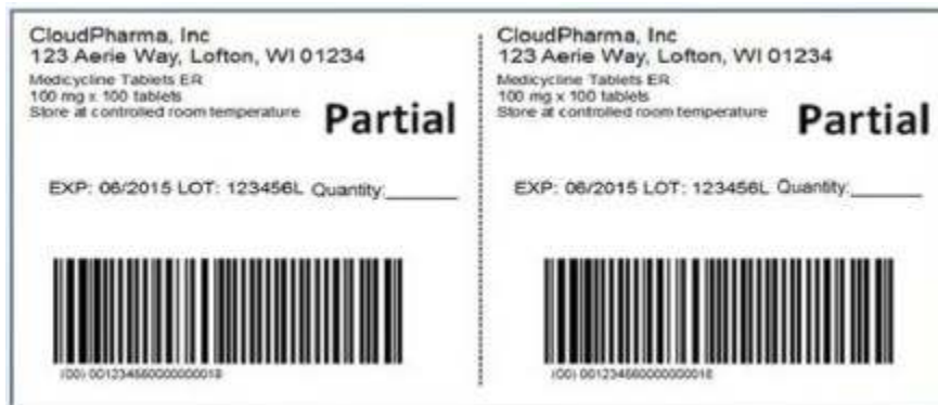
Example Partial Case Labeled with SSCC
