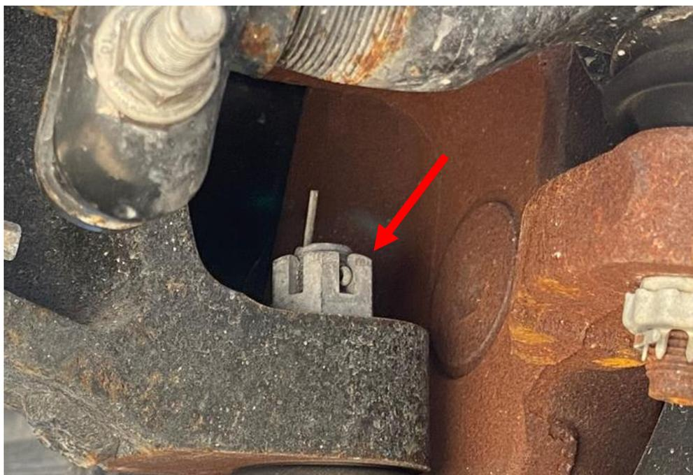
39. As a result of the inability to adjust castor / camber, the Cutaway when in finished form, becomes nothing short of a chore to drive with constant “pulling” or “wandering” on the roadway, difficulty steering, significant premature tire wear and/or uneven tire wear.
