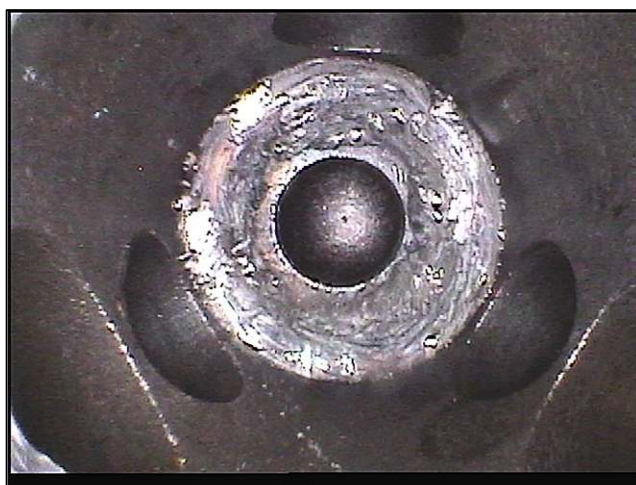
Above: Flashing on the inner diameter of the support tube of an exemplar ARC hybrid inflator.
